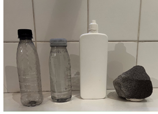
Fig. 3. The objects used for estimating distance using the stereo vision sub-system. From left to right: Textured clear bottle, smooth clear bottle, white bottle, stone.
