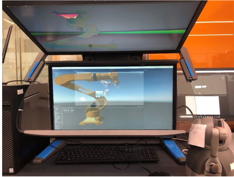
Fig. 1. 3D PluraView stereo display as part of the experimental setup with Touch haptic controller for teleoperating the virtual model of a remote robot-manipulator. The visual scene on the screen shows a combined view of the virtual robot and the stereo view from the remote environment or its emulator.
